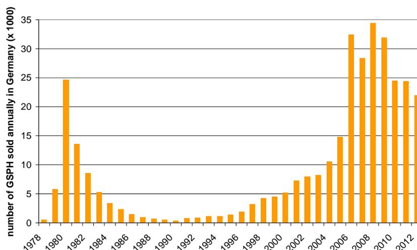
Figure 8: Long-term development of ground source heat pump sales in Germany (both brine and water, 1978-2012) (after annual data from BWP, latest BWP 2013)
