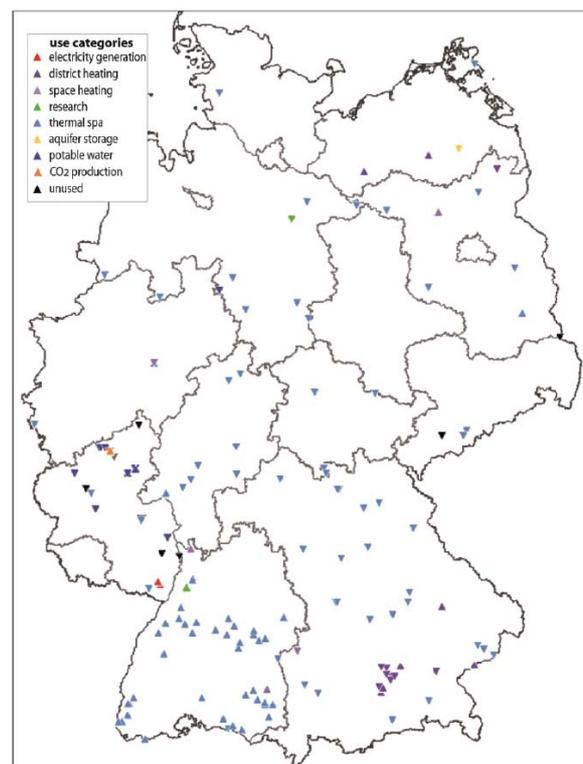
**Figure 5: Installations for geothermal energy use in operation in Germany (from [www.geotis.de](http://www.geotis.de)).**
