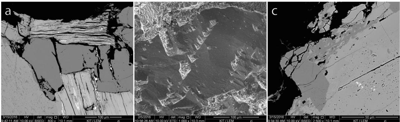
**Figure 1: SEM images (SE and BSE) of the granite sample after 260 °C experiment: (a) disintegrated rock fabric due to chloritization of biotite and quartz dissolution (dark grey); (b) triangular etch pits on the quartz surface; (c) albitization of K-feldspar at the mineral-fluid interface.**
