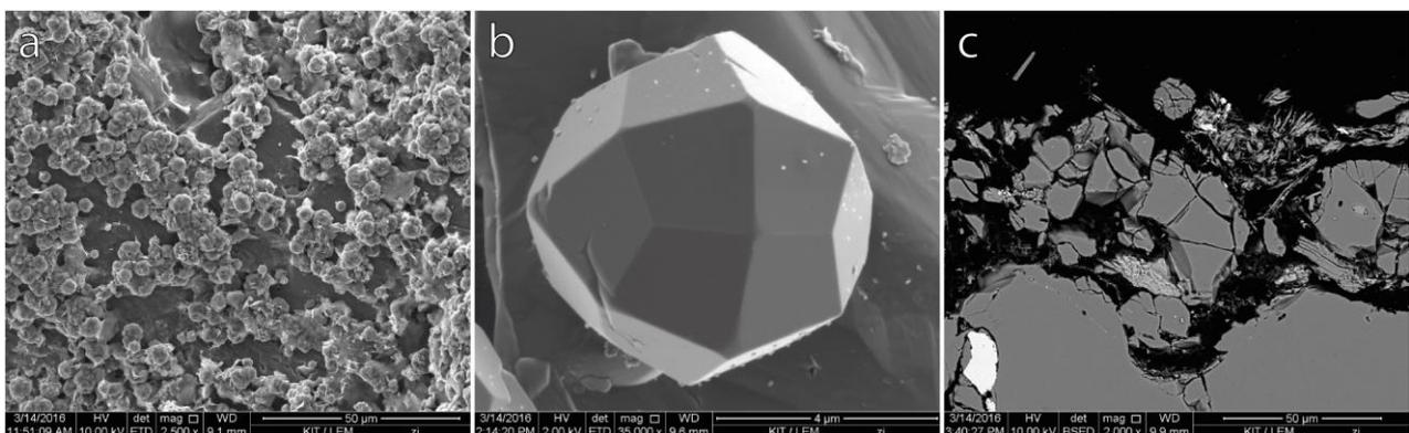
**Figure 2: SEM images (SE and BSE) of analcime precipitation on sandstone sample after 260 °C experiments: (a) sample surface is covered by euhedral analcime (TenSst), (b) spherical analcime on PfSst, (c) BSE thin section image (PfSst) with partly dissolved sandstone matrix, quartz grains and secondary analcime.**
