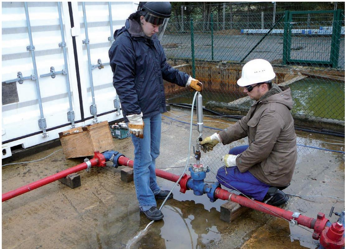
Fig. 20: Fluid sampling to determine the water and gas composition at the Horstberg well
