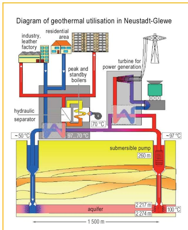
**Fig. 40:** Sketch showing the principle behind the Neustadt-Glewe combined heat and power plant
