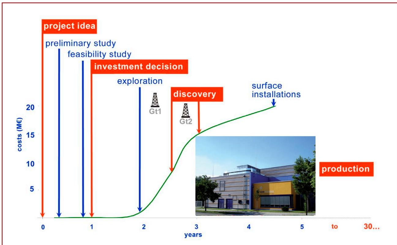
Fig. 10: Different stages of a geothermal energy project: time line in comparison to necessary investments (green line); the size of the investments can fluctuate strongly depending on the nature of the project.
