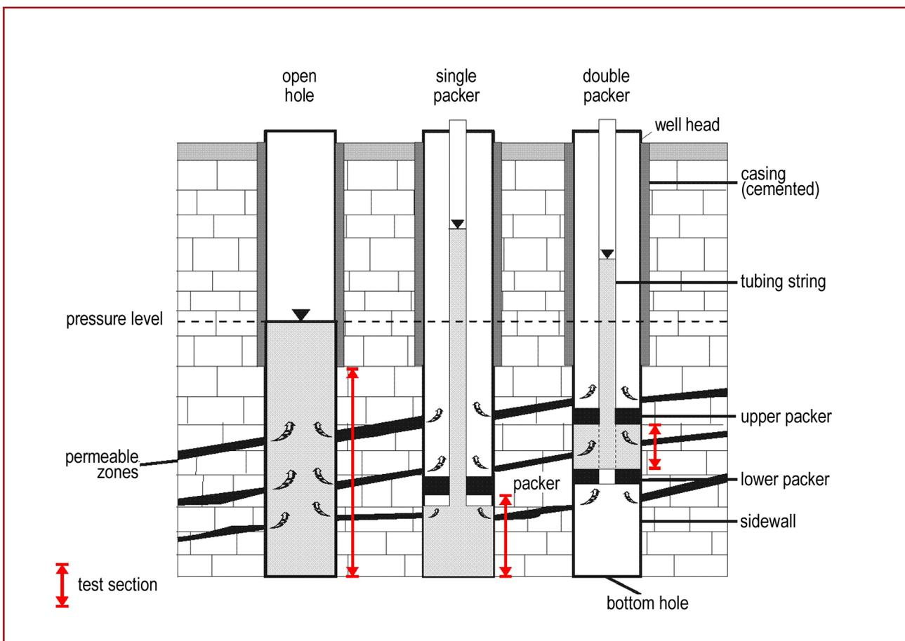
**Fig. 21: Different methods for carrying out hydraulic tests in boreholes (after: NIEDERSÄCHSISCHES LANDESAMT FÜR ÖKOLOGIE & NIEDERSÄCHSISCHES LANDESAMT FÜR BODENFORSCHUNG 1997)**
