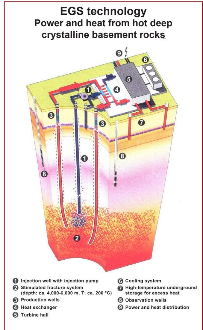
Fig. 12: Diagram showing an enhanced geothermal system (EGS) ([www.geothermie.de](http://www.geothermie.de))
