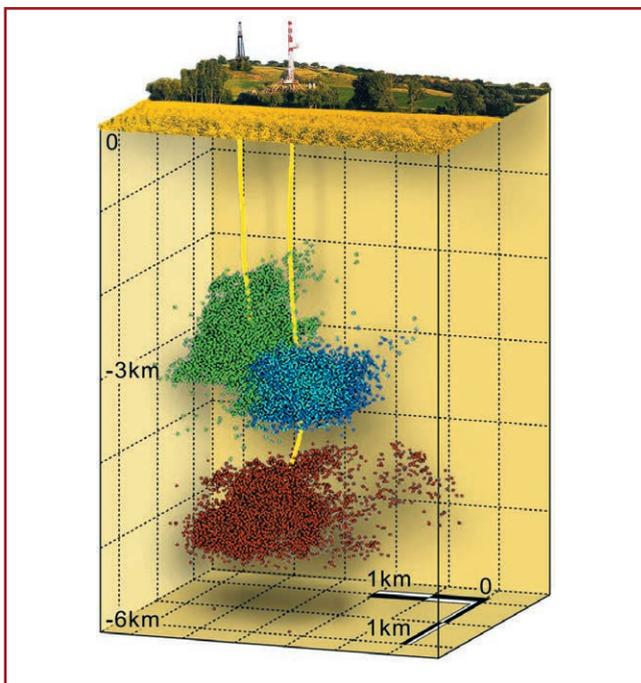
Fig. 16: Hydraulic stimulation in deep wells at the EGS project Soultz-sous-Forêts (France) (WEIDLER et al. 2002): Every dot corresponds to a microseismic event caused by the injection of water; the cloud of dots highlights the artificially created heat exchanger surface.
