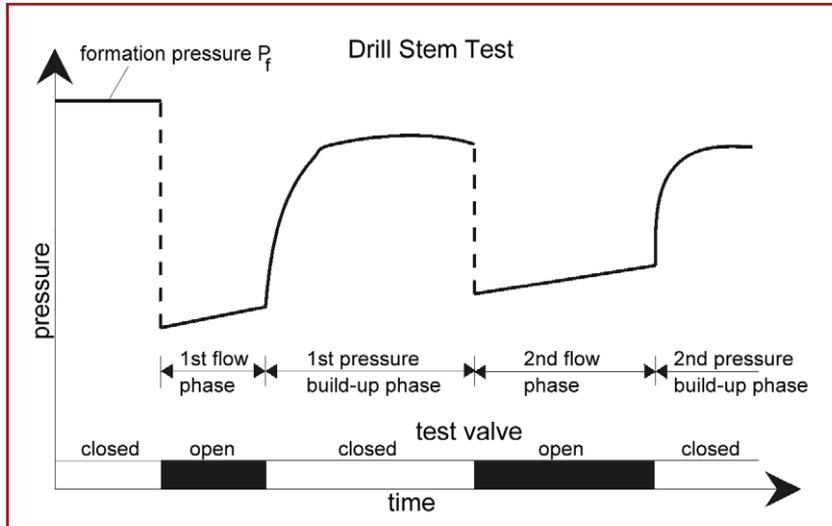
Fig. 25: Typical pressure response during a drill stem test
