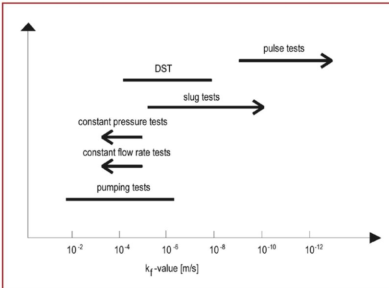
Fig. 22: Application ranges of various hydraulic test methods depending on the hydraulic conductivity (after: NIEDERSÄCHSISCHES LANDESAMT FÜR ÖKOLOGIE & NIEDERSÄCHSISCHES LANDESAMT FÜR BODENFORSCHUNG 1997)
