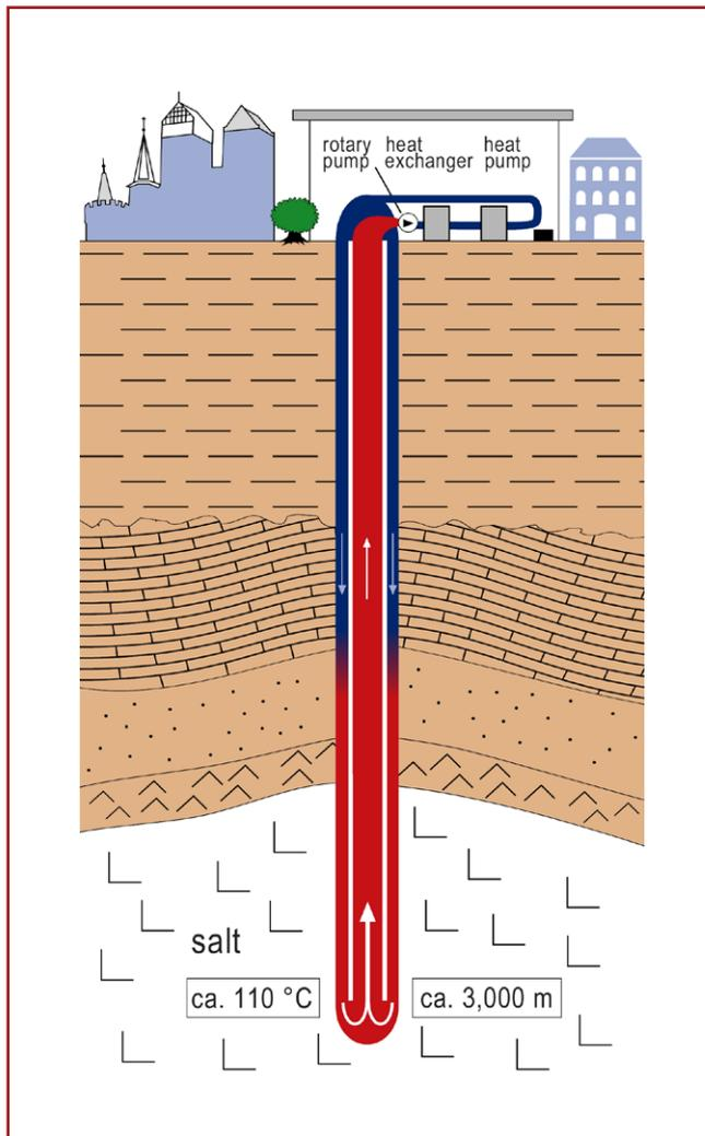
**Fig. 18: Geothermal plant operated by the municipal utility in Prenzlau: Example of a deep borehole heat exchanger (source: Stadtwerke Prenzlau)**
