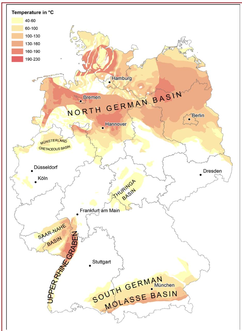
Fig. 28: Overview of regions in Germany considered suitable for hydrothermal utilisation and associated temperature ranges (map adapted from SUCHI et al. 2014). The most important regions are the North German Basin, the Upper Rhine Graben and the South German Molasse Basin.
