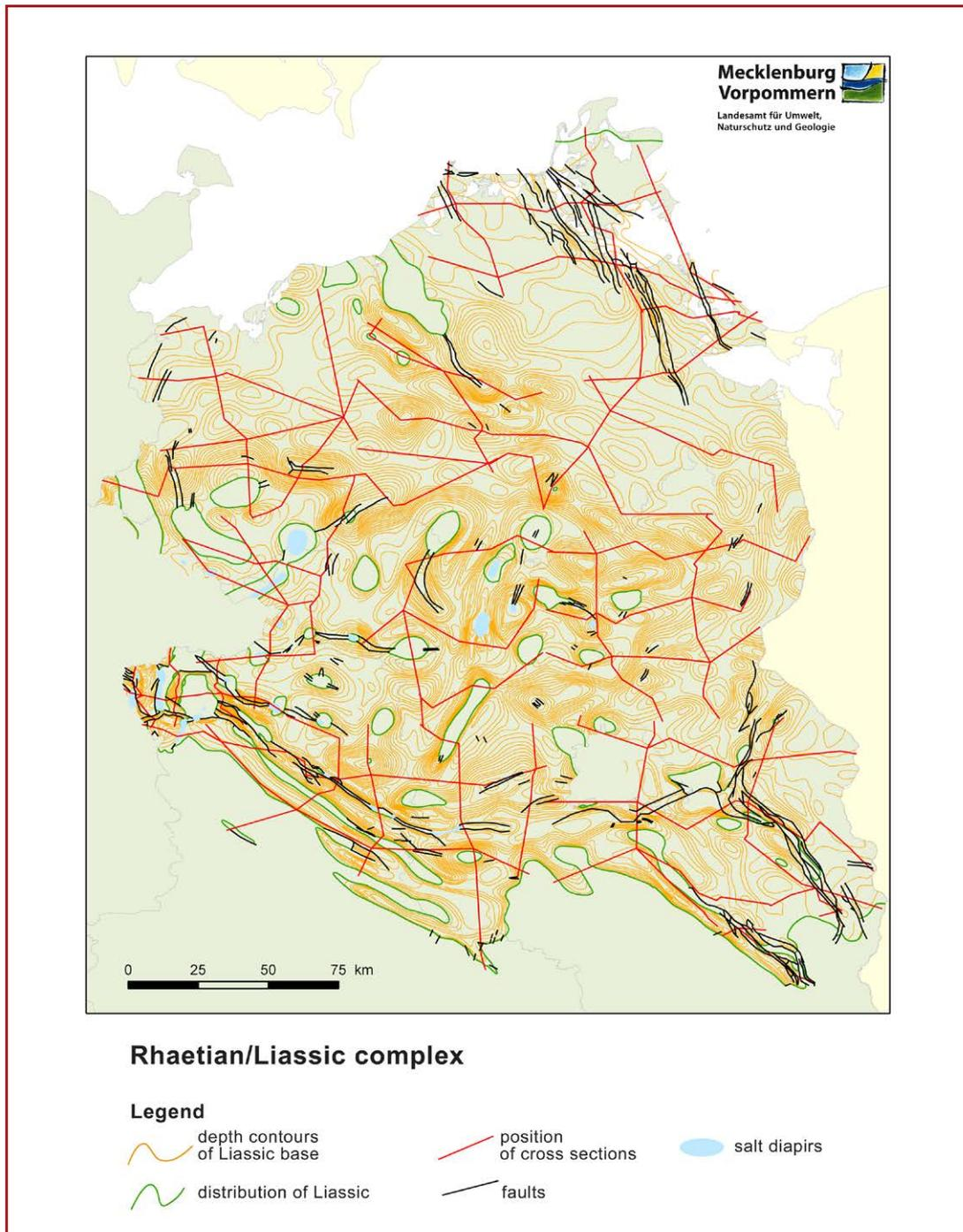
**Fig. 30: Distribution and depth of aquifers in the Rhaetian/Lias complex in northeast Germany. The figure also shows the most important faults and salt structures, as well as the position of cross sections (red) (OBST et al. 2009).**
