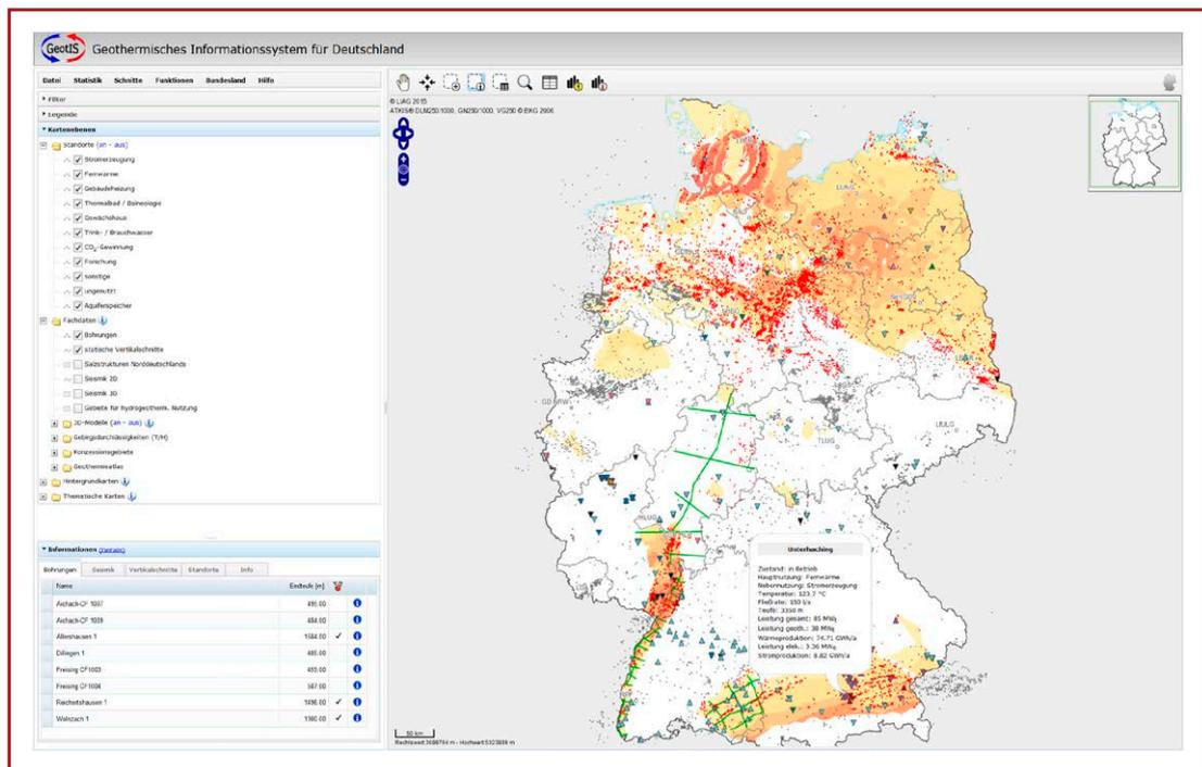
Fig. 27: Screenshot of GeotIS. The geothermal information system offers information on geothermal installations in Germany and comprehensive data for estimating regional potentials of deep geothermal energy.
