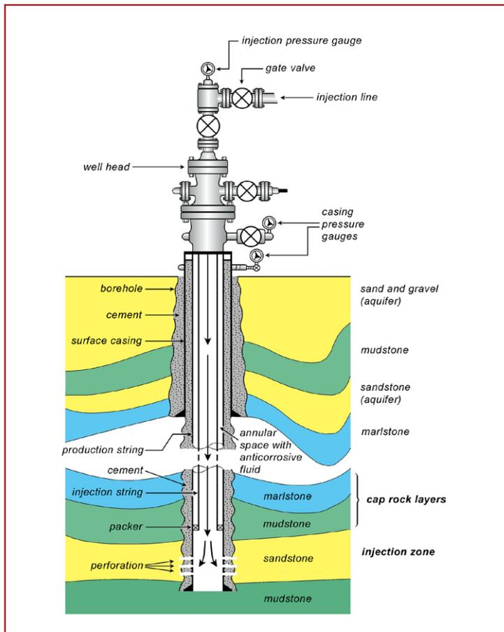
Fig. 8: Diagram of an injection well (modified after OWENS 1975)
