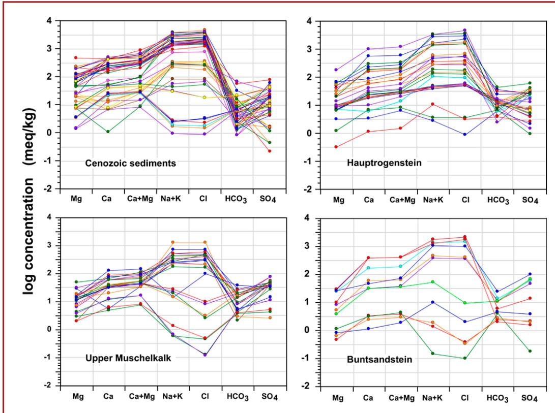
Fig. 34: Hydrochemical properties of waters from potential target horizons in the Upper Rhine Graben (Schoeller diagram) (STOBER & BUCHER 2014)
