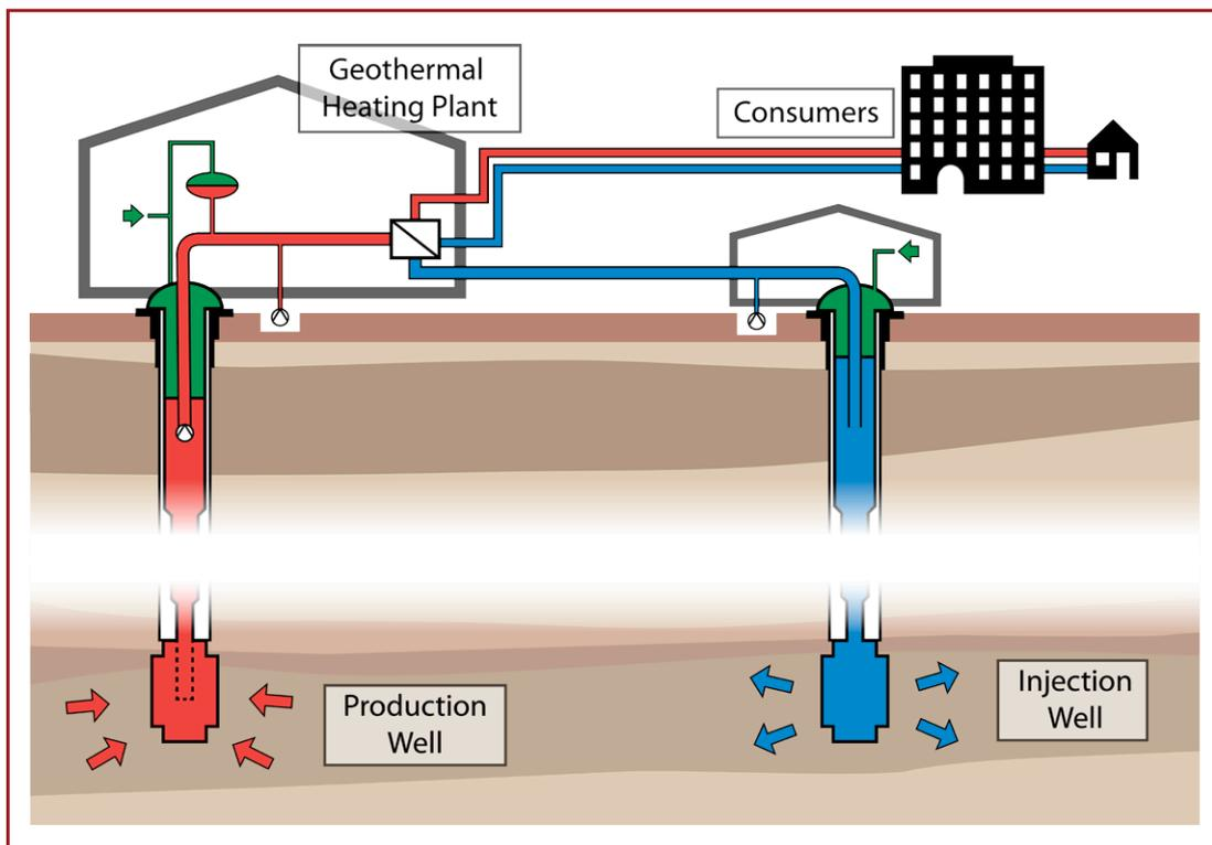
Fig. 4: Diagram of a doublet for hydrothermal utilisation
