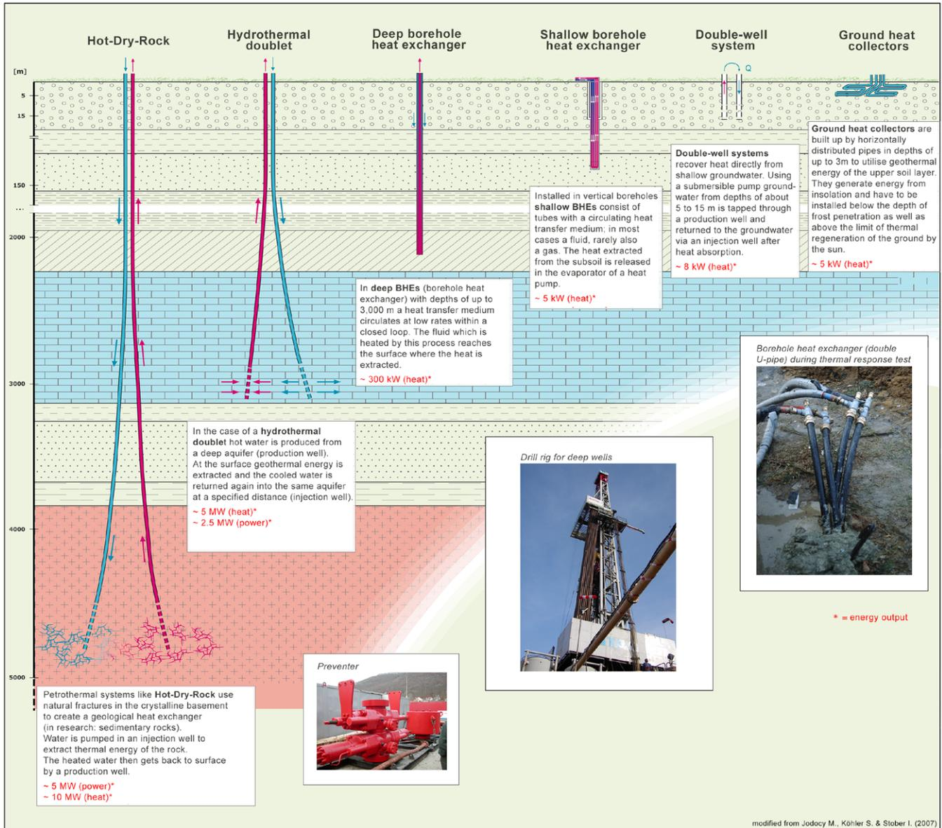
Fig. 1: Examples of different types of geothermal energy utilisation
