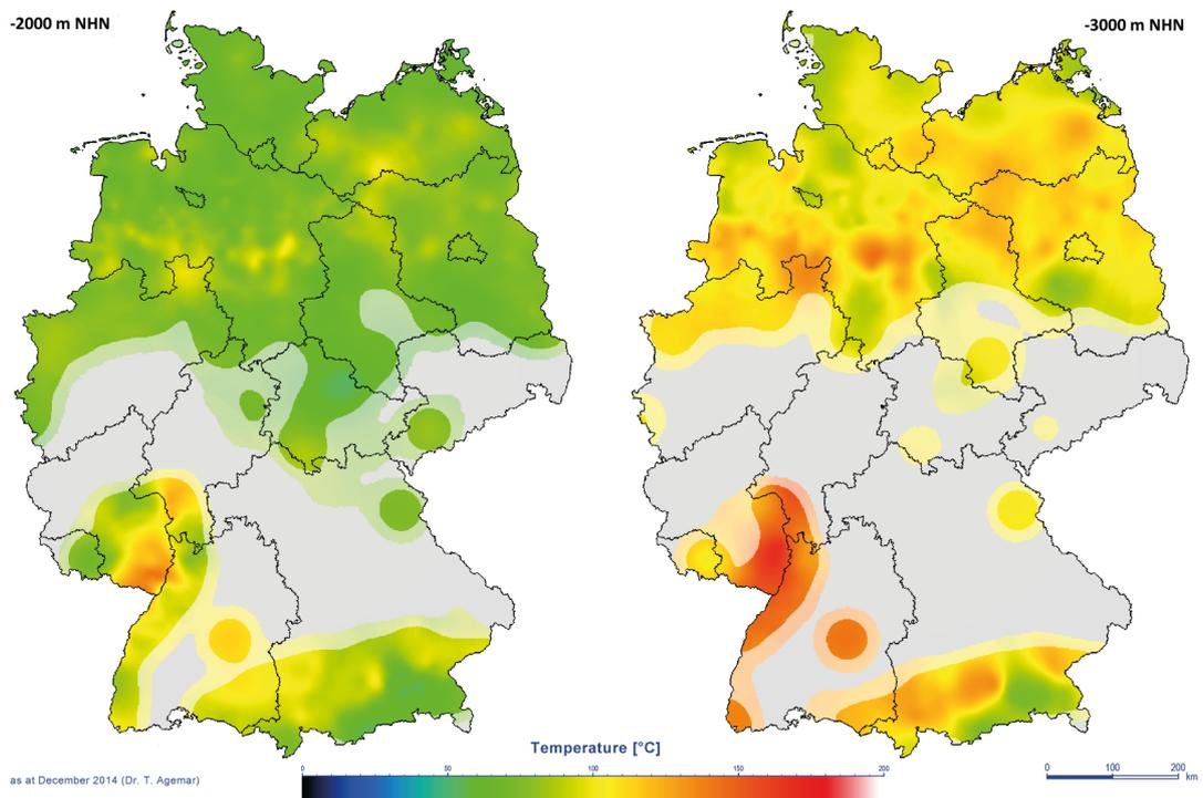
**Fig. 2:** Subsurface temperature distribution in depths of 2,000 m and 3,000 m below sea level. Areas without measured data are greyed out.
