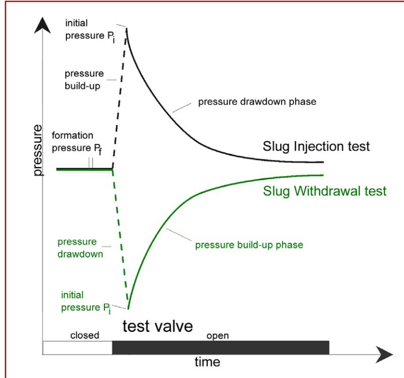
Fig. 24: Typical pressure response during a slug test
