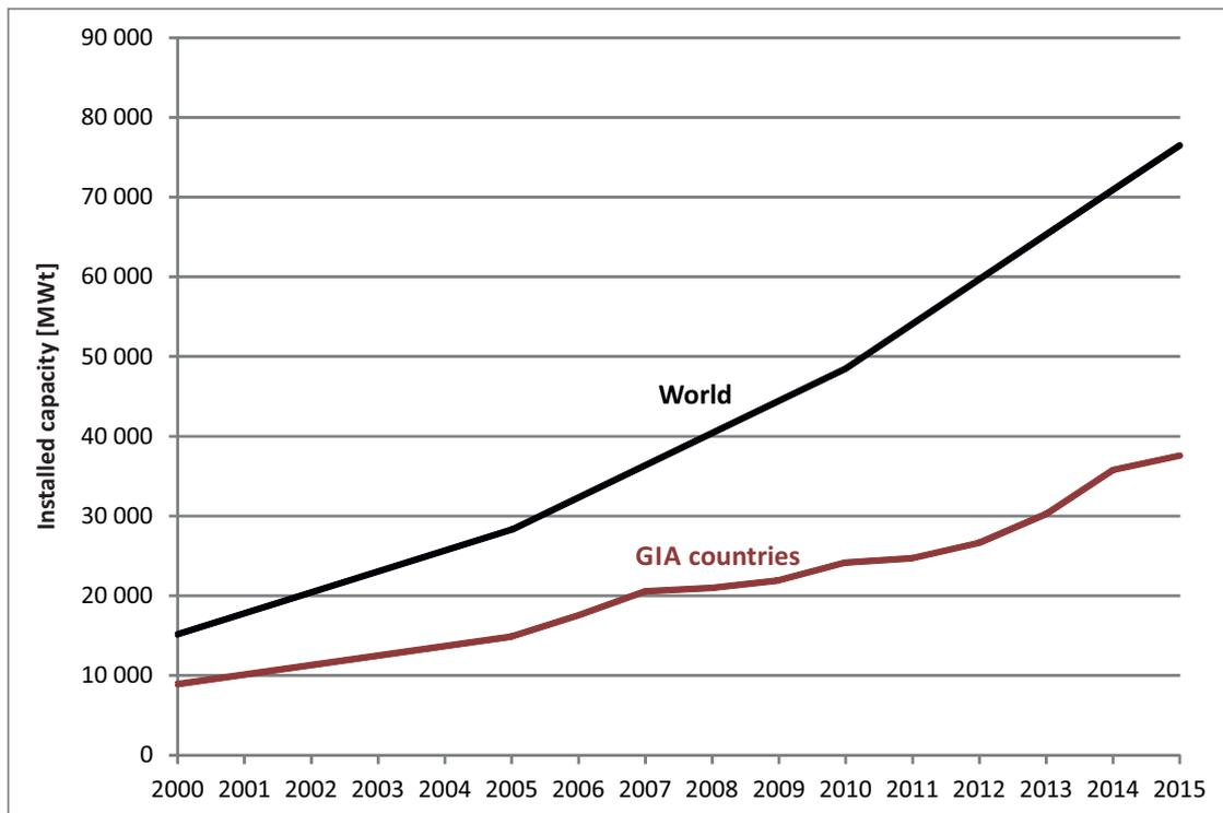
**Figure 10: Installed capacity [MW<sub>t</sub>] of all geothermal heat uses (direct use and GHP use) in GIA countries and worldwide 2000 - 2015.** GIA country data: GIA Annual Reports 2007, 2008 and 2009, and WG 10 country reports 2010 to 2015; world data: Lund & Freeston, 2001; Lund et al., 2005 and 2011; and Lund & Boyd, 2016; 2015: estimated assuming a compound annual growth rate of 7.9%.
