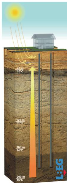
**Figure 9: Principle of GSHP systems using borehole heat exchangers.** The yellow arrow shows the average geothermal gradient. The enthalpy of near-surface systems, indicated by the shallow cavities on the left side, derives mainly from solar radiation. Image: Courtesy of State Authority for Mining, Energy and Geology, Lower Saxony, Germany (LBEG).
